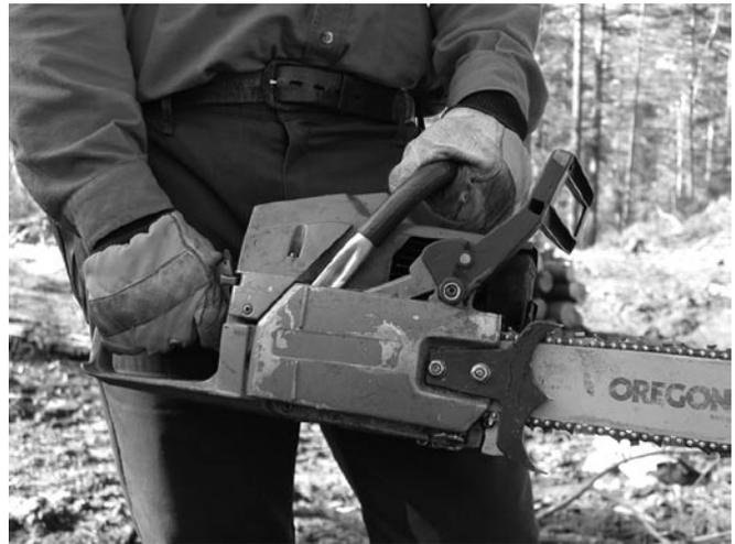
Hold the chain saw with two hands anytime it is running and the brake is not on. Keep the thumb of your left hand wrapped under the forward handle so that the saw cannot easily be pushed back out of your grasp.
