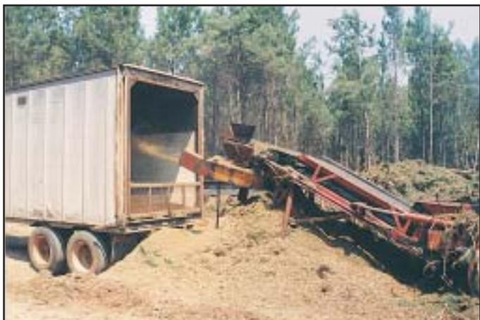
*Finer chips made from tops and limbs are blown from the grinder into a large enclosed truck for transport to a boiler or storage facility.*
