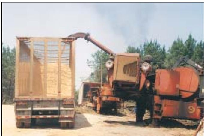
*Chips are blown into trailers and trucked to the purchasing mill.*
