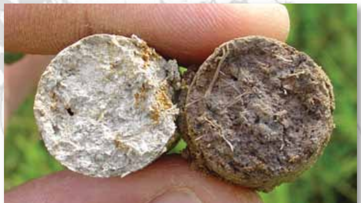
These cores contrast poorly-drained soils (left, 95% gray) with well-drained (right, 0% gray).
