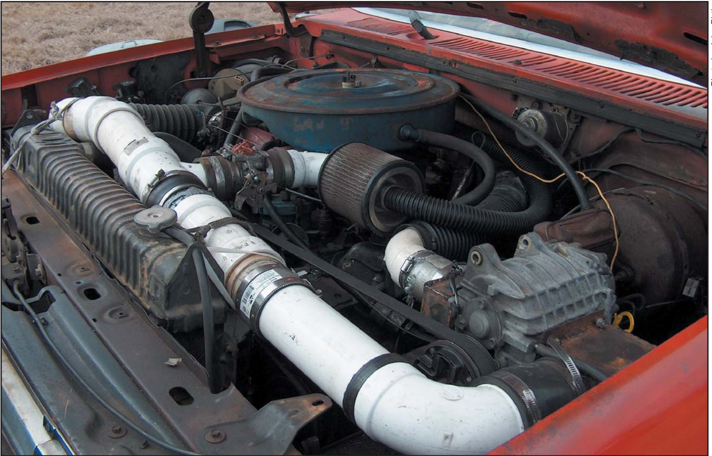
Synthesis gas – produced from solid biomass by a technology called gasification – passes through a series of filters in front of the hood, and directly to the carburetor where it burns almost as well as gasoline.
