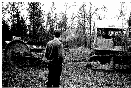
The drum chopper can be used on steeper terrain than shearing.
