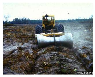
bedding requires an area sufficiently free of debris and vegetation to allow forming the beds, it is usually combined with other mechanical treatments.
