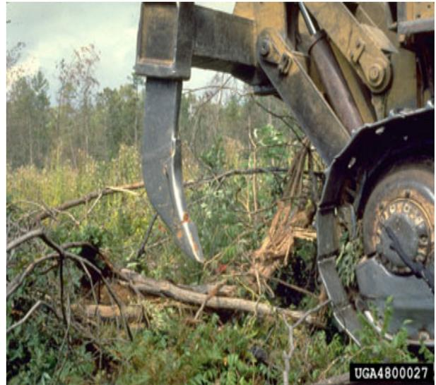
**EQUIPMENT:** In-row subsoiling is performed using a single- or multiple-shank instrument pulled behind a large farm tractor or similar mechanized equipment. The subsoiling shank must be a minimum length of 18 inches in order to rip the soil to a depth of 15 inches. A tree planter foot does not qualify as a subsoiling instrument.
