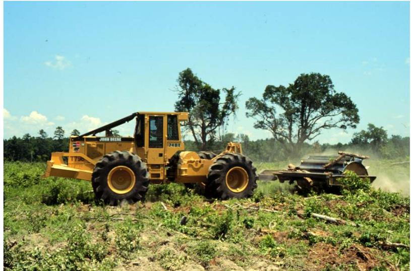
For smaller vegetation, a straight blade is satisfactory and a smaller tractor or rubber-tired skidder may be used. The crawler or skidder must be capable of pulling a conventional roller drum chopper filled with water. The drum should be 8 - 10 feet wide and equipped with sharp blades.
