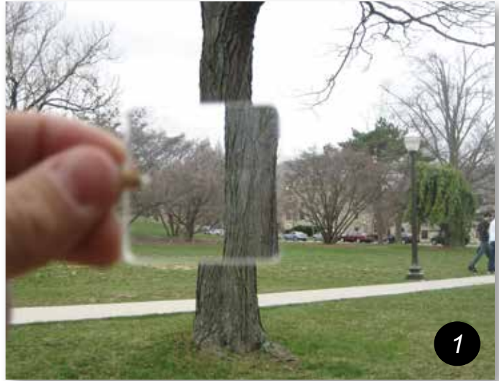
A tree is considered 'in' if the offset section of the tree overlaps the bole as viewed with the prism.
