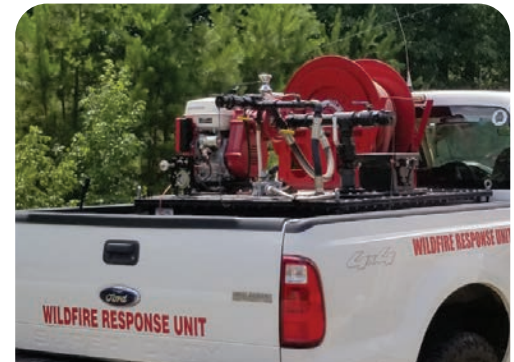
Franklin pumper mounted on truck
