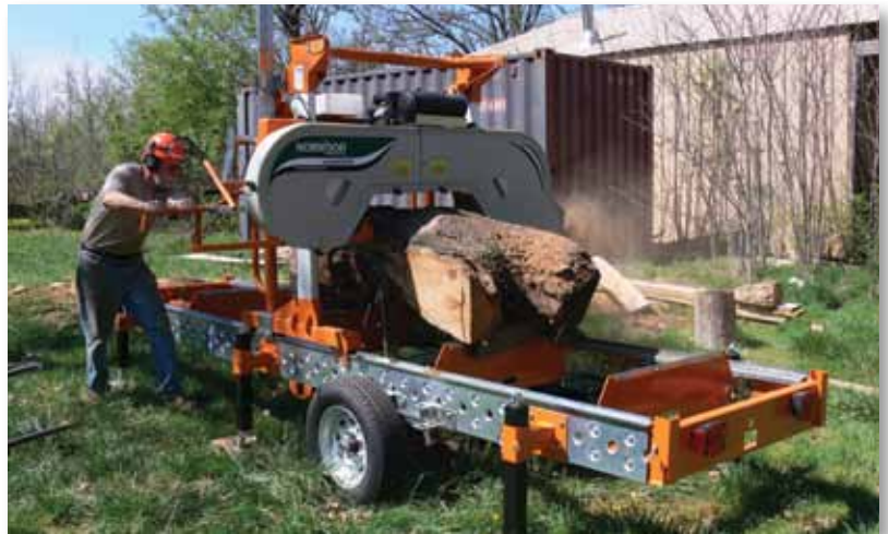
The same cherry log on the sawmill. The mill’s ability to handle a variety of shapes and sizes makes it especially useful for salvaging logs and lumber.
