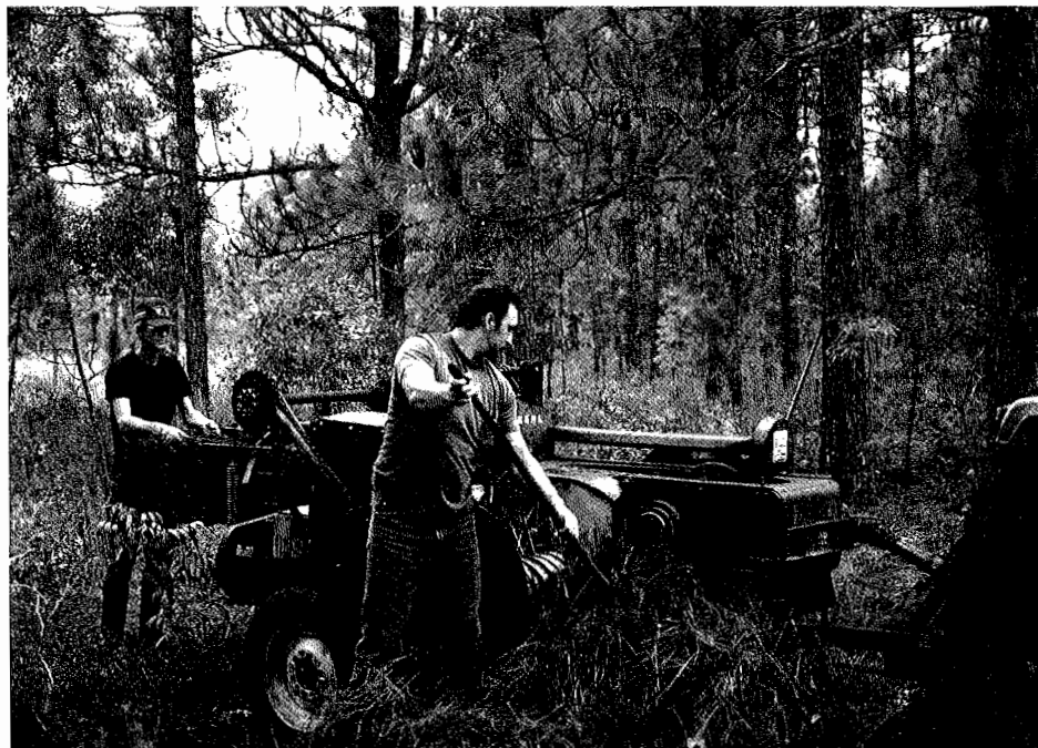
Baling is done by modified hay balers or hand presses (box balers). Both methods require that the straw is hand fed.
