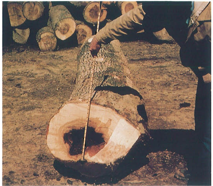
What may look good standing may be of little value at the mill. Here is a good sample of the scaling defect "BUTT ROT."
