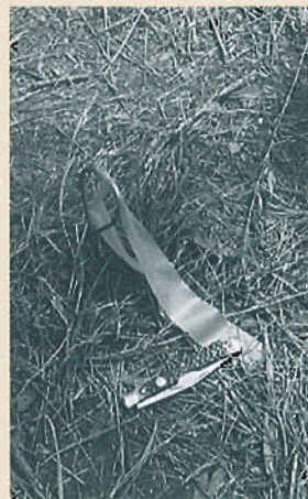
Witness trees are used to locate the plot center, which is marked by a metal pin.
